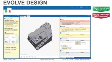
EVOLVE Design imports CAD models to create tolerance simulations, proving that specific datum points will be accepted or rejected.
